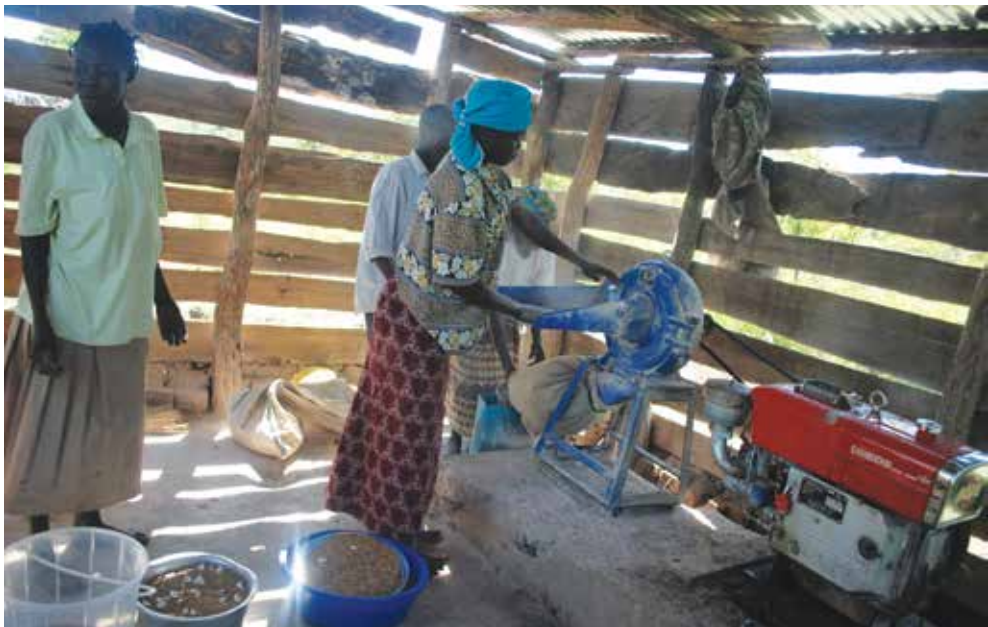
Too Okema Livelihoods group tests the milling machine with maize grain, millets, cassava and sorghum to make flour for porridge and bread.
